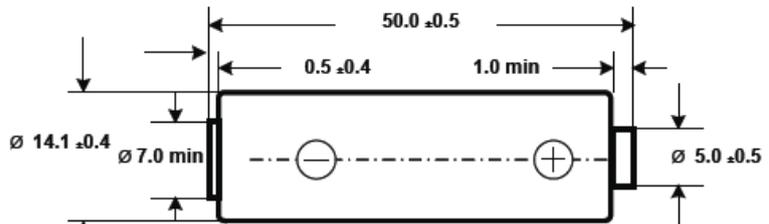
Dimensions are in millimeters and include label.
